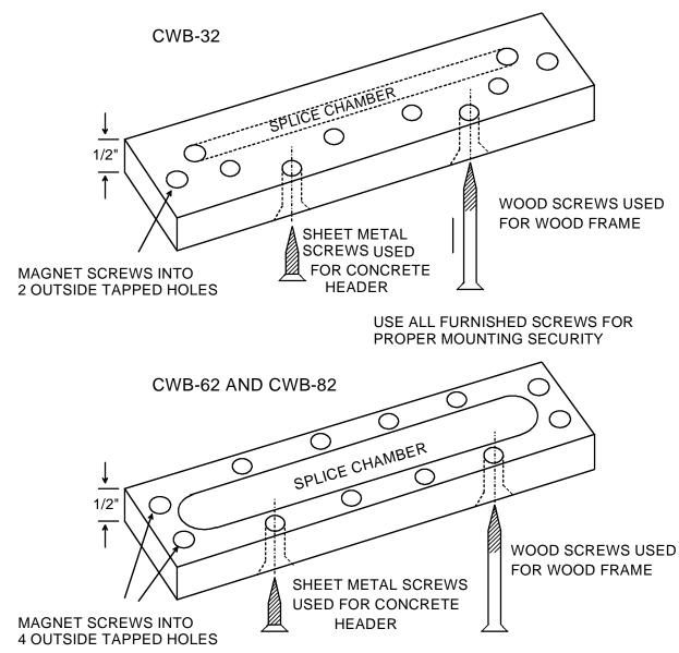
FIG. 12: WOOD FRAME AND CONCRETE HEADER BRACKET
